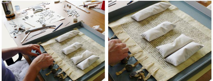
One side of the box should open in order to comfortably pull out the tray. Due to the assembly on the tray, the documents and especially the delicate seals are protected from skidding around and can still be submitted for use.
