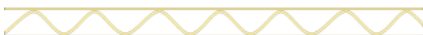
Fig. 3c: Construction of E-flute corrugated board, (3.0 mm) laminated on both sides with cardboard (190 g/m 2 ).
